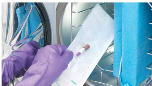
Figure 10. Placing the BI in the sterilizer
